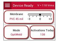
**Activations Log:** The "Activation Today" button displays the number of weld cycles performed on that calendar day. Pressing this button will open the tool log, where a history of weld cycles can be reviewed.
