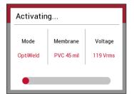
Once the tool settings are complete and accurate for the membrane type and thickness being installed, the tool is ready to weld.
