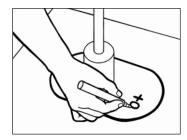
At the end of the weld cycle, place a magnetic cooling clamp on the plate, and mark the energy setting on the membrane for reference.
