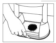
Set the energy setting to the lowest setting that you think will provide a complete bond (e.g. level #0) and weld the first plate.
