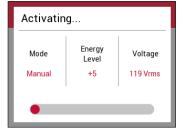
Press the trigger on the handle to activate the weld cycle.
