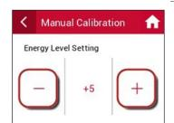
Adjust the "Energy Level" to the next higher setting, and repeat the test weld process until all five plates are welded with increasingly higher energy levels.
