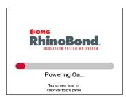
When first powering up the RhinoBond tool, the main screen will show a status bar indicting tool startup progress. If necessary, you can calibrate the touch screen at this time. To do so, touch this screen once to begin the calibration process (see below).
