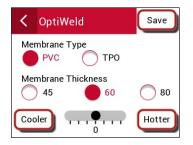
From the "Device Ready" screen, press the "Membrane" button and select the type (TPO or PVC) and thickness (45, 60, 80 mil) of the membrane you are installing.
