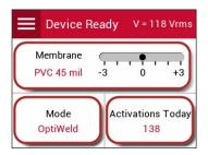
When set in OptiWeld mode, the "Mode" button displays OptiWeld. Membrane type and thickness and fine adjust set-tings are also displayed. Pressing the "Mode" button allows users to toggle between "OptiWeld" and "Manual" operating mode.
