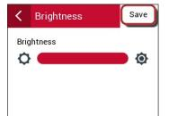
Select the "Display" button to adjust the screen brightness. Press the sun icons on either side of the bar to increase or decrease the screen brightness.
