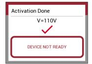
When the weld is complete, the RhinoBond tool will emit a beep, provided that the sound is turned on (see Page 11), and display the "Activation Done" screen.
