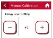
The "Energy Level" button displays the current energy setting that will be delivered to the RhinoBond plate.
