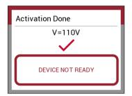
Once the weld is complete, the RhinoBond tool will emit a beep, provided that the sound is turned on (see pg 11) and display the "Activation Done" screen.
