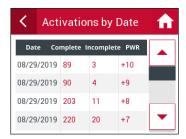
The table will show the date, welds completed (check mark) and welds with an error message.
