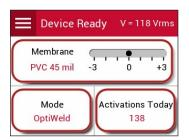
From the "Device Ready" screen, press the "Mode" button, and select the "Manual" option.
