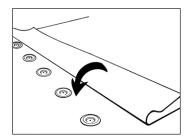
To calibrate the tool, place at least five (5) plates on insulation about 10-inches (25 cm) apart, and cover the plates with a piece of membrane from the project.
